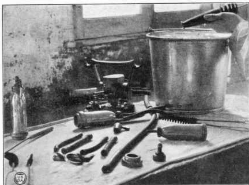
FIGURE 7.—The machines should be taken entirely apart and washed thoroughly with brushes and hot water containing washing powder
